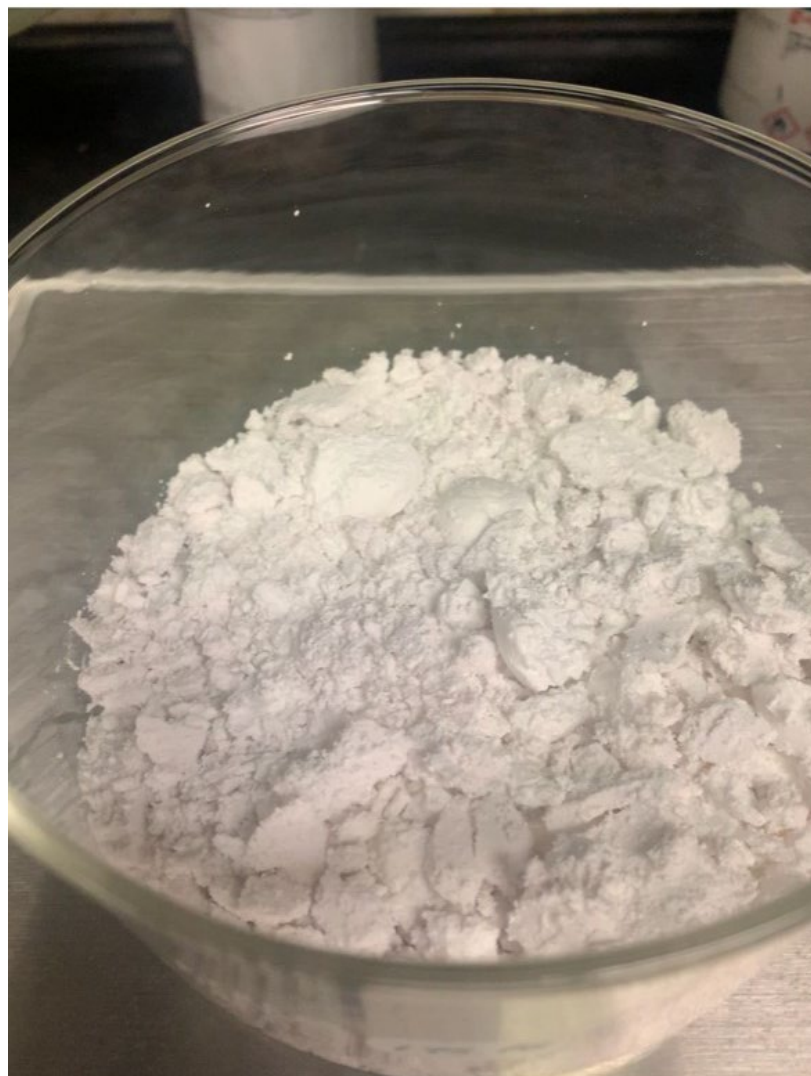
Figure 2. Photograph of polyureas obtained from stirring of 50 g/L TDI (80:20 2,4-:2,6) in distilled water for 14 d:
