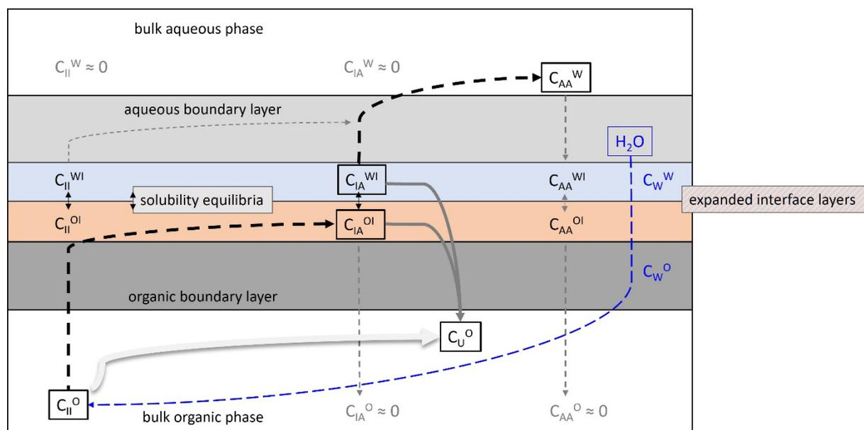
Figure 2 - Schematic representation of the main processes taking place at the water-organic interface.
