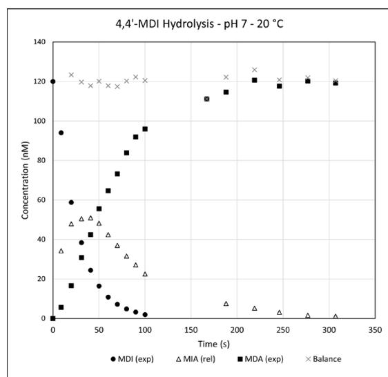
Figure 1 - Two-step hydrolysis of MDI in water.
